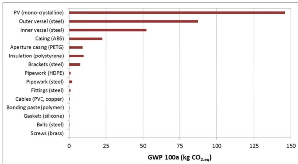
**Fig. 3.** Contribution of each component/material to the total GWP 100a of one PVT module.
