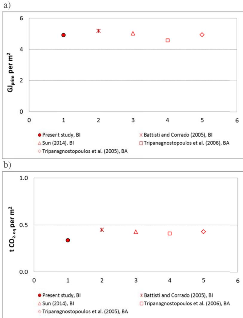
Fig. 5. Comparisons in terms of: a)  $GJ_{prim}$  and b)  $t CO_{2,eq}$  per  $m^2$  of PVT module.
