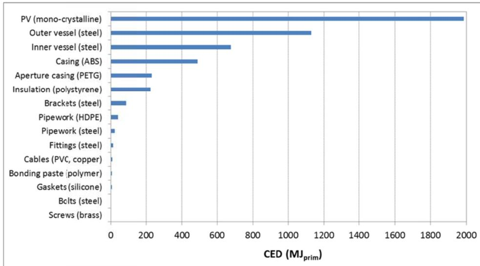
**Fig. 2.** Contribution of each component/material to the total CED of one PVT module.
