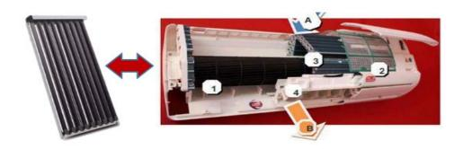
Solar vaccum tubes collector is integrated in a thermal loop which is composed by an air/water heat exchangers situated inside the habitat. Calories are transferred from solar collector to the habitat throught the air/water heat exchangers by natural convection or by forced convection with a pump.
