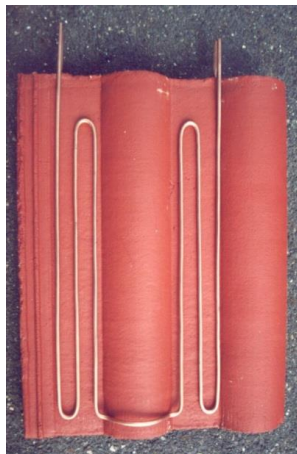
Fig. 5. The tile element design
