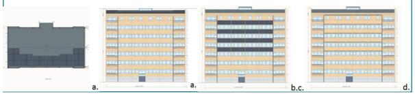
Fig. 2. (a) I Design Variant: roof 40° (roof and facade layouts), (b) II Design Variant: parapet 90°, (c) III Design Variant: parapet 45° and (d) IV Design Variant: sun shading 0°
