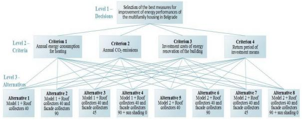
Fig. 4. Structuring of problem of the selection of the best measures for improvement of energy performances of the multifamily housing in Belgrade
