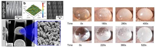
Fig. 8. (Left) Micrographs with relevant length scales and structures in single-tier and multitier structures for icephobicity: (a) etched Si nanocones, (b) etched SiO<sub>2</sub> nanopits, (c) etched SiO<sub>2</sub> micropillars, and (d) etched Si micropillars/nanotextures with the nanotexture depicted in the inset image (Schutzius et al. 2015). (Right) Icing process of a water droplet on a plain copper surface (top) and a nano-fluorocarbon coated surface (bottom) (Wang et al. 2012).
