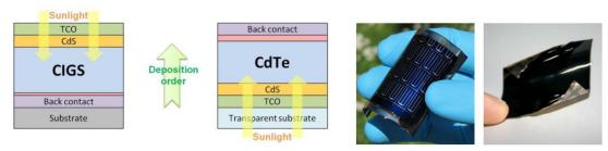
Fig.4. Principle configuration build-up and photos of flexible CIGS (nos. 1 and 3 from left) and CdTe (nos. 2 and 4 from left) thin film solar cells (Buecheler et al. 2011).
