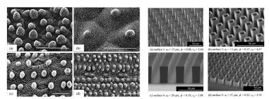
Fig.7. Micromorphologies for water-repellent leaf surfaces of (a) Nelumbo nucifera and (b) Lupinuspolyphyllos (scale bars =  $50 \mu m$ ), and (c) Gladioluswatsonioides and (d) Sinarundinaria nitida (scale bars =  $20 \mu m$ ) (left four photos) (Hsu et al. 2011). Images of four artificially fabricated hollow hybrid superhydrophobic surfaces (scale bars =  $50 \mu m$ ) (right four photos) (Dash et al. 2012).
