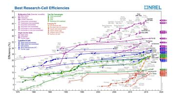
Fig. 2. Best research-cell efficiency timeline (enlarge digitally to see details) (NREL 2016).
