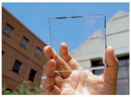
Fig.3. Solar harvesting tuned to absorb specific non-visible wavelengths of solar radiation and letting visible solar radiation pass straight through (Mourant 2014).
