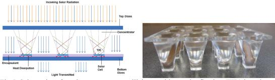
Fig. 5. Schematics of a solar concentrator utilizing total internal reflection (TIR) in order to guide the incoming solar radiation to the active solar cell parts (left) and actual concentrator element array made of polyurethane (right) (Baig et al. 2015).
