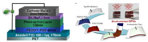
Fig.6. (Left) Device structure of a flexible polymer solar cell (Heo et al. 2011). (Right) Schematics depicting a brush painting process of preparing brush-painted flexible organic solar cells. The inset photo shows the flexibility of the brush-painted flexible organic solar cells (Kang et al. 2014).
