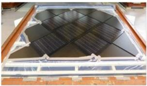
Fig. 11. GS Integra Line SP (configuration B) with a greater number of PV modules (Andenæs, 2016).
