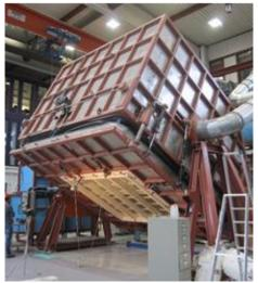
Fig. 6. Large-scale turnable box for rain and wind tightness testing of sloping building surfaces (RAWI box) (Breivik et al., 2013).
