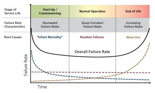
Fig. 7. The "Bathtub curve" of failures occurring in solar PV modules (Sirkin, n.d.).
