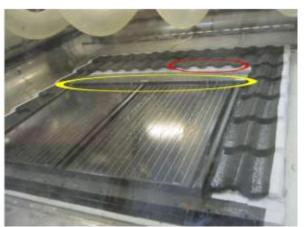
Fig. 8. Sample roof with integrated DuPont Gevity modules inside the RAWI box during testing, the colored ellipses denote leakage points (Breivik et al., 2013).
