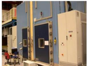
Fig. 3. Specially customized large-scale vertical building envelope climate simulator consisting of a sample field installed between the exterior and interior climate chambers (Jelle, 2013).
