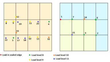
Fig. 13. Leakage points observed during rain tightness test of BIPV roof tile at 15 degree inclination (Andenæs, 2016).
