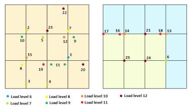
Fig. 12. Leakage points observed during the rain tightness test of the BIPV roof tile at a 30 degree inclination (Andenæs, 2016).
