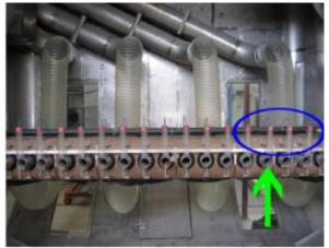
Fig. 5. The boom inside the RAWI box which delivers wind-driven rain across the sample area. The blue tubes on top (blue ellipse) supply water down to the transparent vertical cylinders (blue ellipse) where it hits the air stream that blows out of the air tubes (green arrow) and is blown onto the sample area (Breivik et al., 2013).
