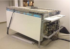
Fig. 4. Accelerated climate ageing of roof samples in a combined horizontal UV, temperature and water spray ageing apparatus.
