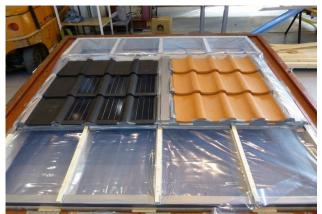
Fig. 9. Heda Solar (left) and Monier Nova (right) tiles mounted in the substrate frame (Andenæs, 2016).
