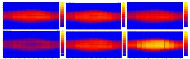
Figure 5: Incident solar radiation charts (kwh/m²/yr) for alternative massing configurations
