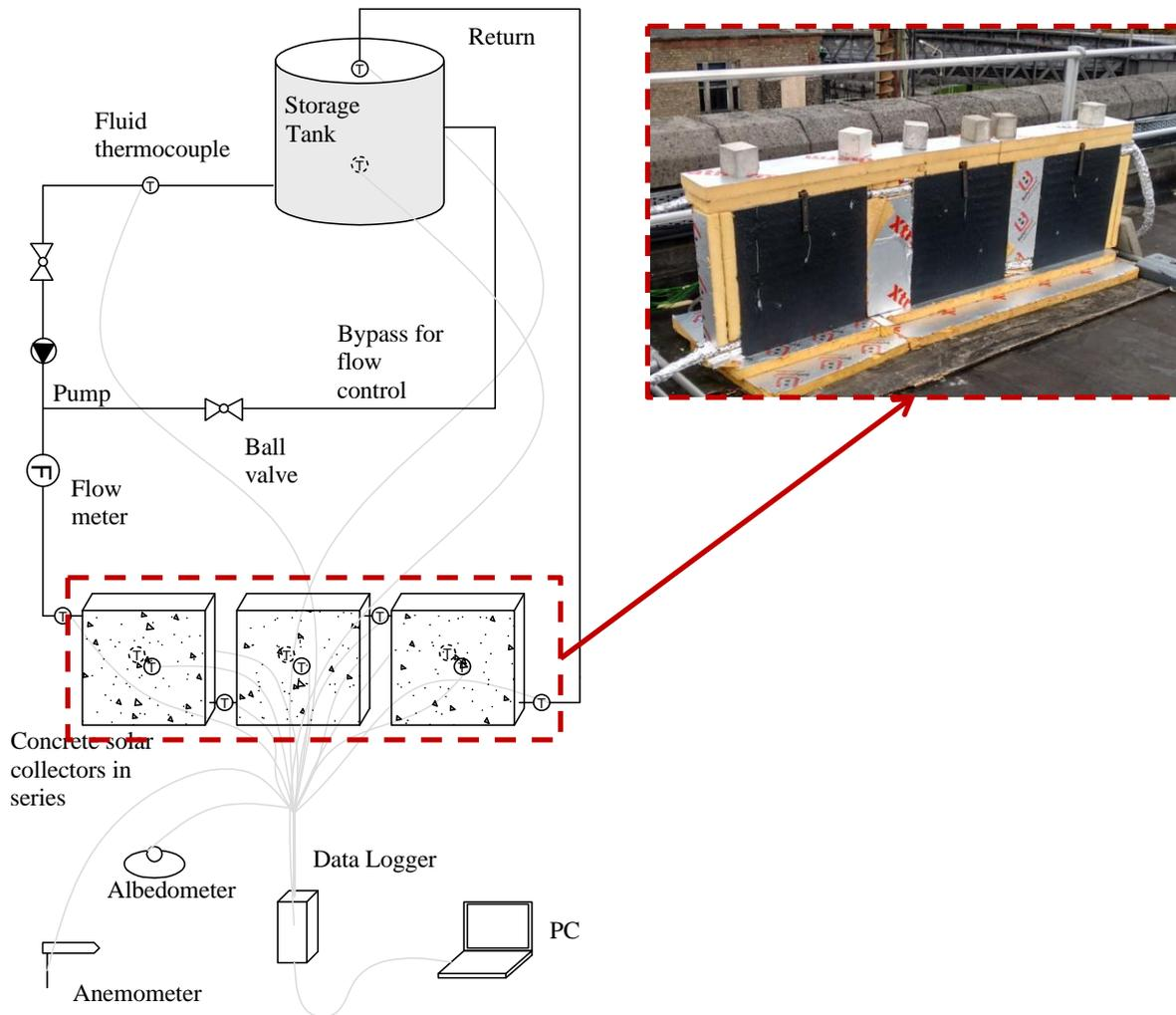
Figure 2. Experimental set-up of the concrete solar collectors (Dublin, Ireland).
