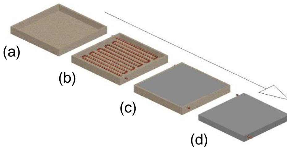
Figure 1. Concrete solar collector construction process (left to right)
