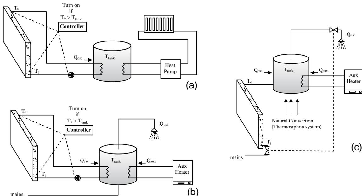
Figure 5. Heating systems suitable for concrete solar collectors.
