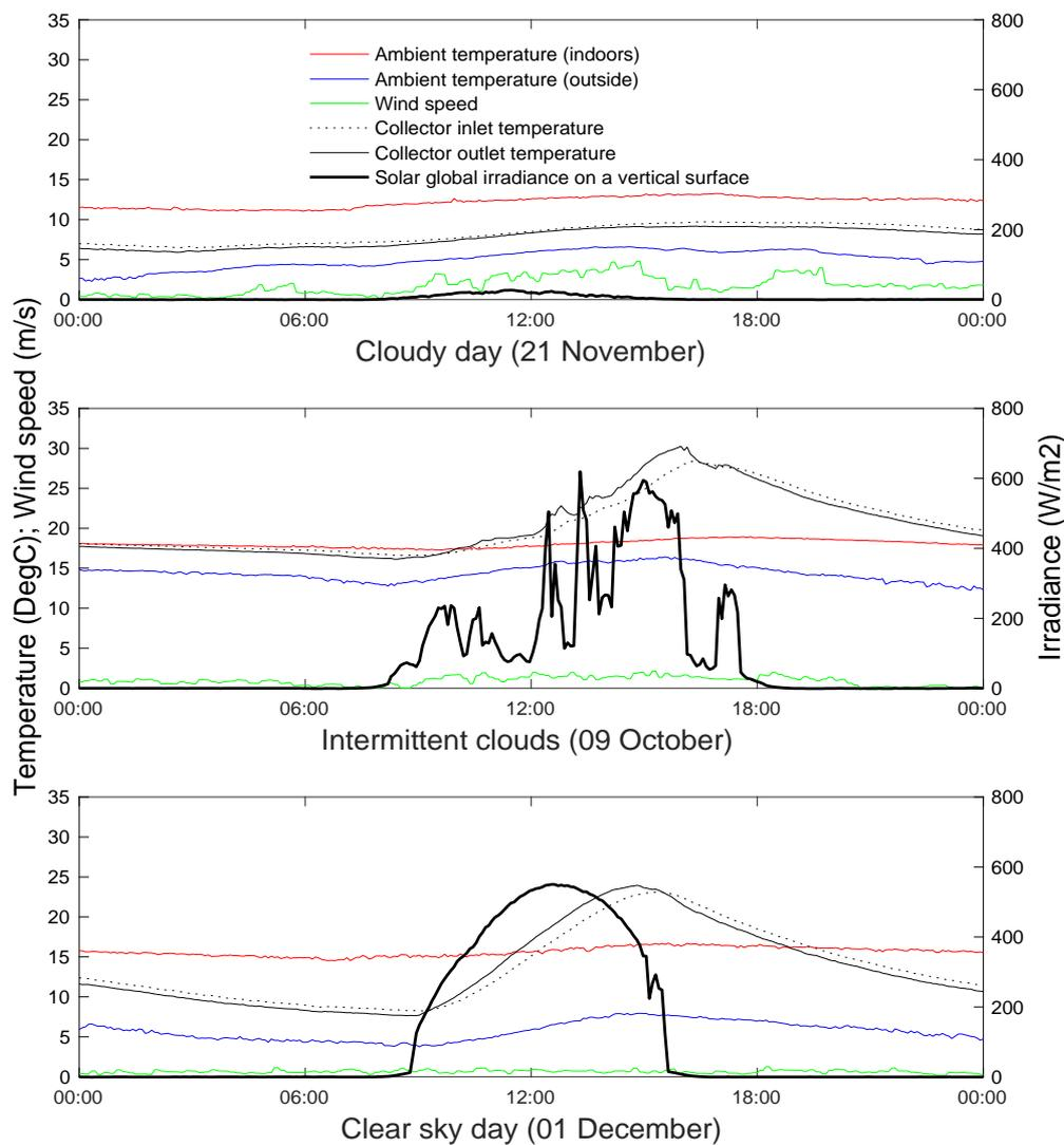
Figure 3. Concrete solar collector inlet and outlet temperatures for three example days
