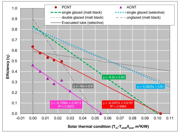
Figure 5: Comparison of instantaneous efficiency of Senergy solar water heater prototypes against other flat plate solar collector benchmarks
