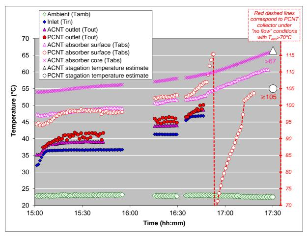
Figure 4: Measured inlet, outlet, absorber and ambient temperatures for both collectors under highest inlet temperature conditions
