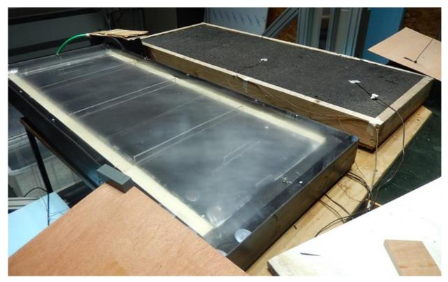
Figure 1: Senergy PCNT (left) and ACNT (right) solar water heating collectors
