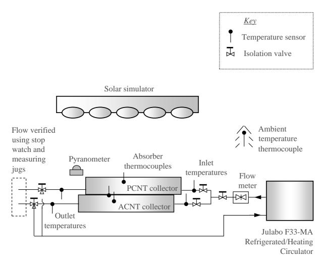
Figure 2: Schematic detail of test facility and instrumentation (two collectors, side by side)
