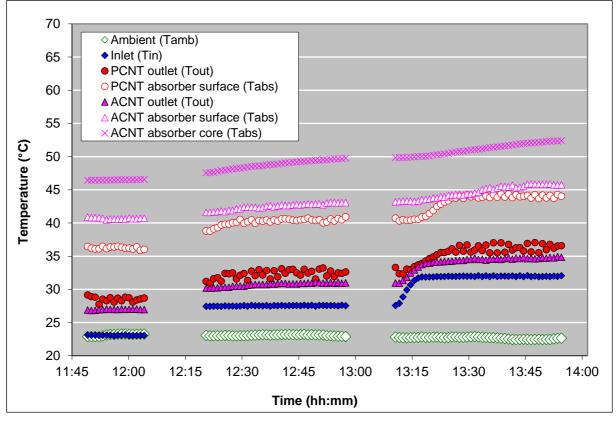
Figure 3: Measured inlet, outlet, absorber and ambient temperatures for both collectors under lowest inlet temperature conditions
