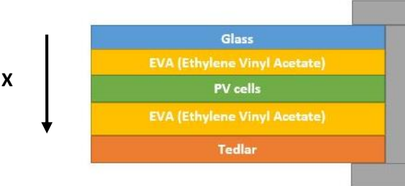
Fig.1. Layered structure of PV laminates with frame
