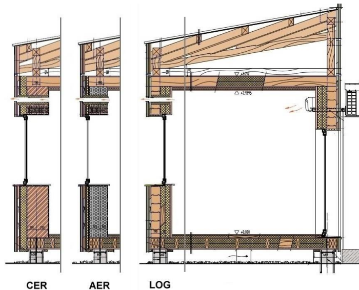
Fig. 2. Cross-section of test buildings' wall envelopes.
