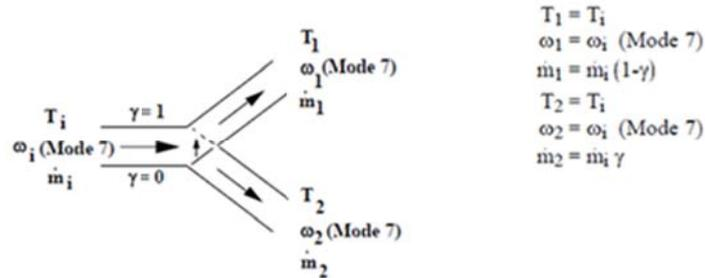
Fig. 3: Flow diverter operation
