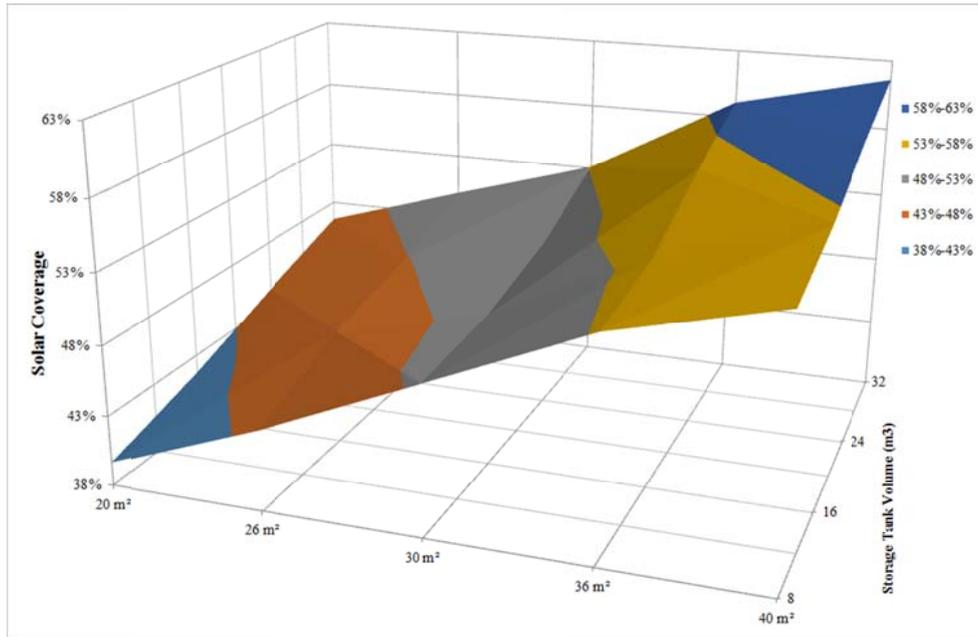
Fig. 5: Seasonal Solar Coverage for roof integrated flat plate collector options
