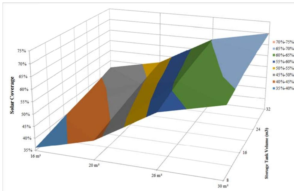
Fig. 6: Seasonal Solar Coverage for façade (16-20m<sup>2</sup>) and roof integrated (26-30m<sup>2</sup>) vacuum tube collector options
