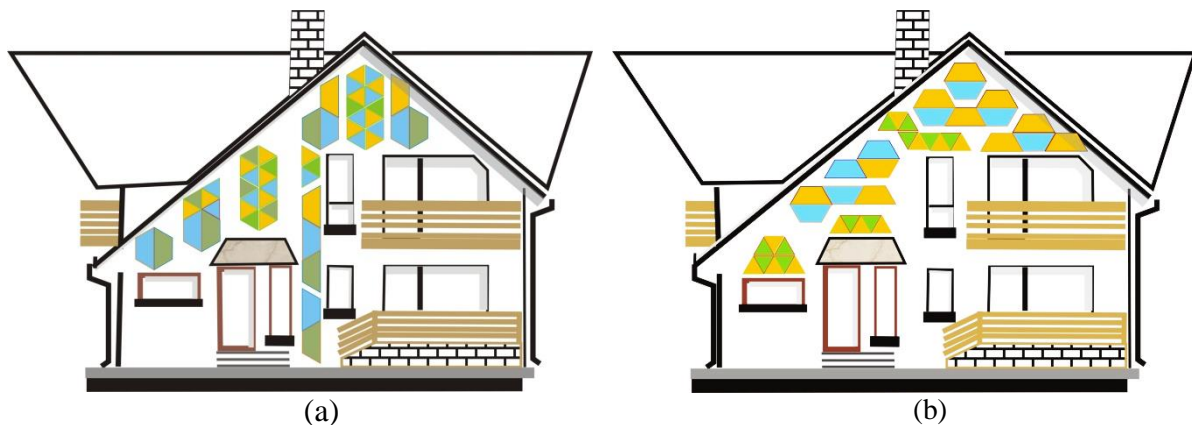
Fig. 1. Solar-thermal facades using groups of triangle solar-thermal collectors and trapeze collectors with (a) „portrait” mounting and (b) „landscape” mounting
