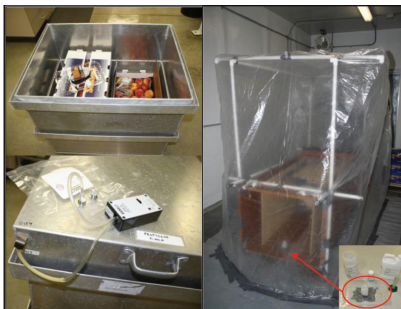
Figure 1. Standard recommended application of 1-MCP (0.5 μL L -1 , 0 °C, 24h) in a sealed 330 L volume aluminum tank (left), and the novel application technique, in a forced air cooler (0.5 μL L -1 , 0 °C, 24h) fitted in a 4000 L volume tend (Right).
