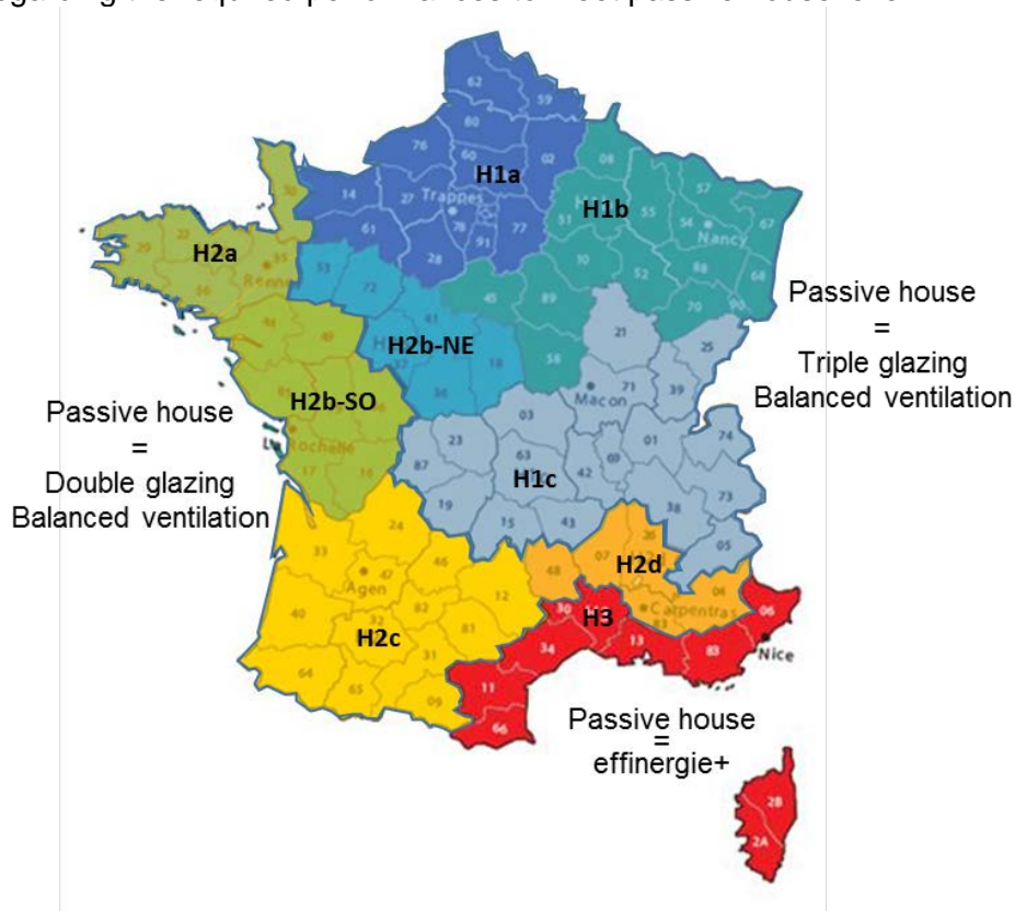
Figure 36: French climatic zones and segmentation for different passive house variants [Pouget 2014]
